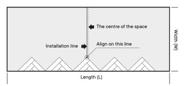
Lay the triangles with the long side towards the starting wall. Place the tip of the middle triangle exactly on the installation line. Make sure the subfloor is laid in advance and that the installation line remains visible.
