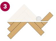
Cut the triangle along the marked line. Depending on the type of saw you use, it may be useful to disassemble the triangle before cutting.
