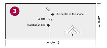
Draw the installation line. Start at the centre of the room. Draw the line parallel to the X measurement for the distance.
