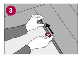
Push the 5G release tool forward. The 5G disassembly pin pushes back the flexible sole and releases the strip for disassembly.
