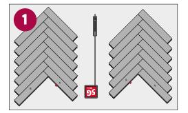
Once a strip is clicked, it is not possible to pick it up by hand. Use the 5G disassembly pin together with the guide block to disassemble the strip.
