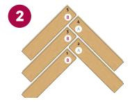
Place the strips accurately in the order indicated by the numbers on the strips. Be sure to check the joints between all the strips.
