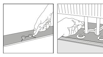
Drill holes twice the diameter of the radiator pipes. Remove a piece of the strip with a knife or a saw. Place the strip on one side of the pipes and the removed piece on the other.
