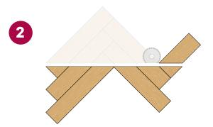
**Excess pieces of the starting triangles:** Separate the excess material from the starting triangles. Use it to close the gaps towards the finishing wall. Use the remaining pieces of strips 1, 2, etc. in order and cut them to size if necessary.
