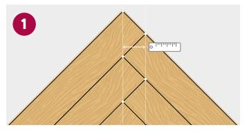
Measure the distance between the two straight lines.
