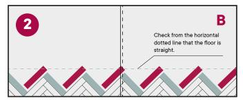
Place **B-strips** and cut the rightmost piece to size.
