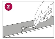
Insert the 5G disassembly pin into the hole of the guide block. Insert the guide block into the groove of the strip.
