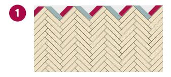
This alternating placement of **A-strips** and **B-strips** is continued throughout the room. It is important to regularly check whether::
