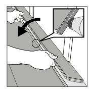
Remove the connecting element as shown. Use a suitable glue to join the strips. Press wedges between the glued strip and the wall.
