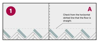
Place **A-strips** to connect all the triangles. The connection between the A-strip and the triangle should be inspected carefully. You should not be able to feel any protruding edges.
